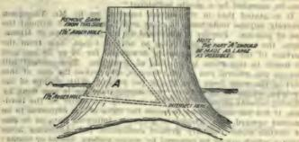
Fig. 10.—Blast Holes in Stump.
